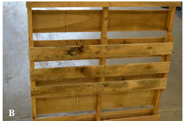
Figure 12 Representative photos of grade 2. (A) Top deck boards (B) Bottom deck boards (With AFTS installed on trailer)
