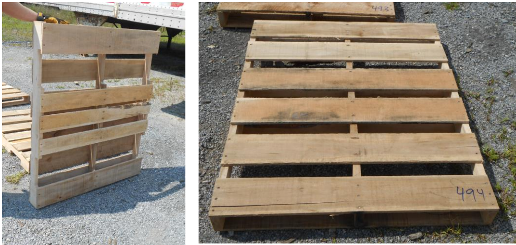
Figure 1 Back and front view of the used three stringer hardwood pallet (GMA Pallet)
