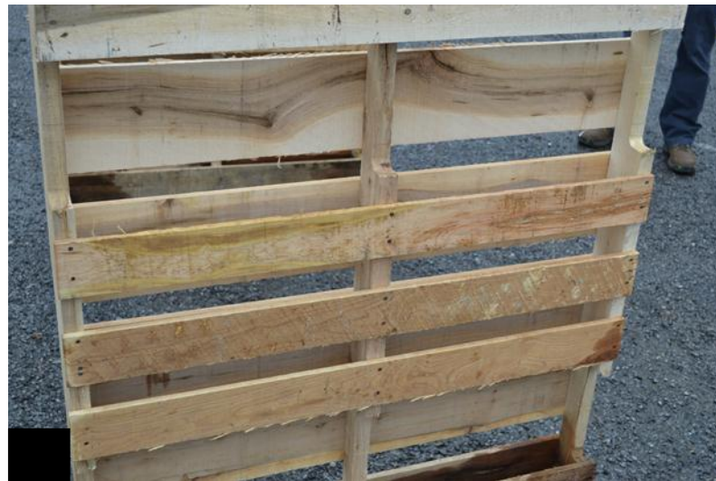
Figure 10 Representative photos of grade 0 (little to no visible mold growth). (A) Top deck boards, (B) Stringers, (C) Bottom deck boards.
